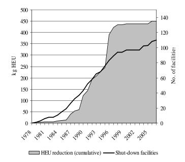
FIG. 2. Shutdown HEU-fueled research reactors and associated HEU consumption (kg) (cumulative) 1978–2007
