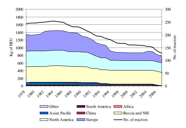
FIG. 1. Operational HEU-fueled research reactors and associated HEU consumption (kg) 1978 – 2007
