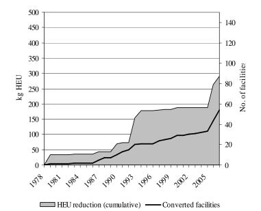
FIG. 3. Converted HEU-fueled research reactors and associated HEU consumption (kg) (cumulative) 1978–2007
